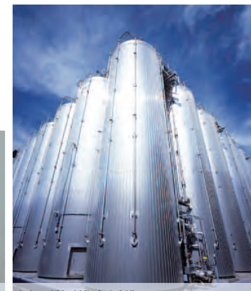
超级不锈钢制酱油酿造罐 Soy brewing tank made of super stainless steel
